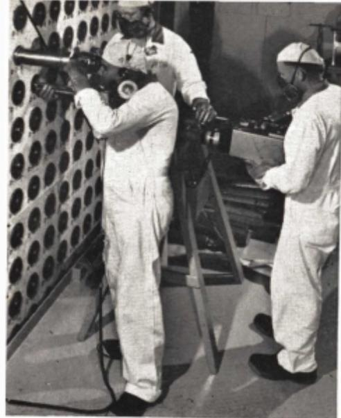
Technicians prepare to remove radioactive samples from face of reactor.
