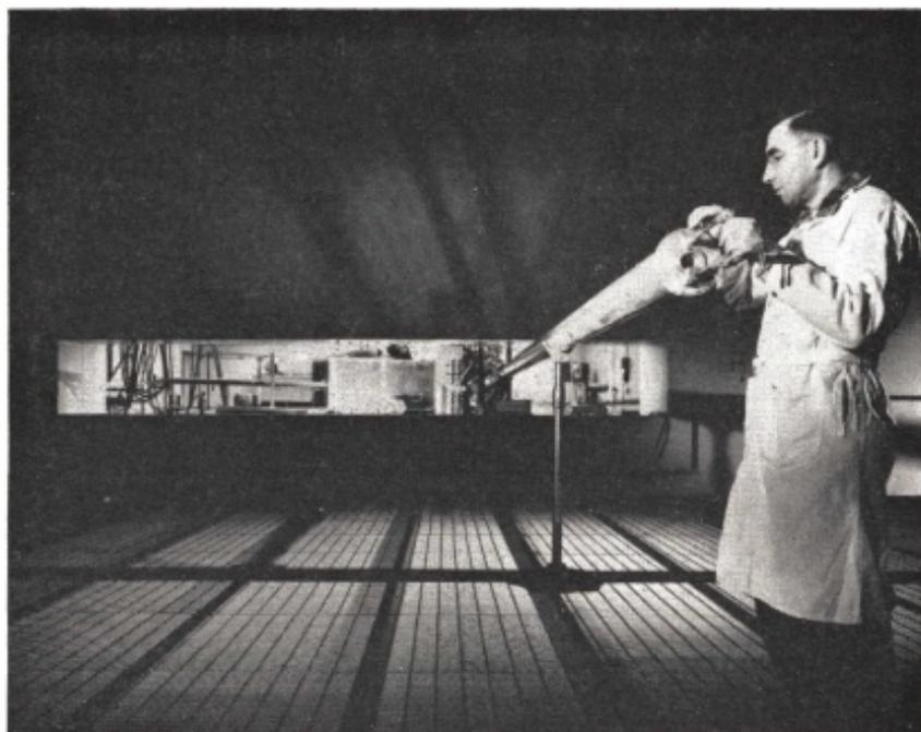
Here is shown a thirty-foot beam pipe leading from a small eighteen-inch cyclotron which produces three mev protons. The protons strike a metal target to produce an intense beam of neutrons. Of course no person is permitted in this area when the apparatus is in operation.
