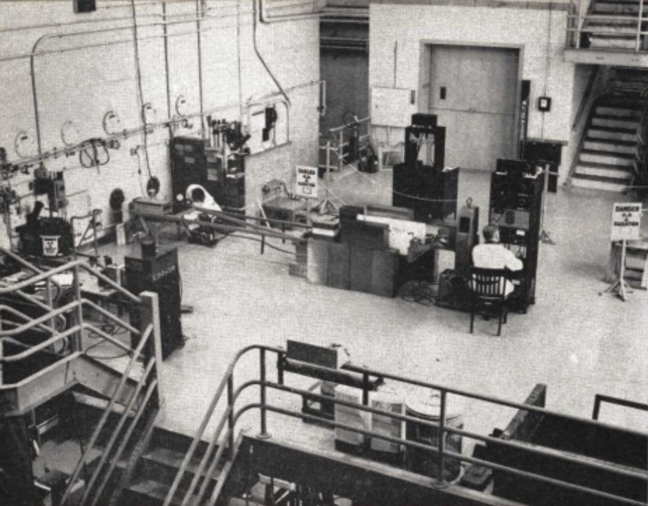
A collimated beam of neutrons is allowed to stream out of the reactor, and is measured by the counting device shown in the center of the area.
